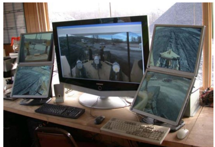
Operator is able to monitor each camera view, independently, on one of four large screens, allowing for safe efficient production. Actual photos from PROVIX IP cameras at Kinross
